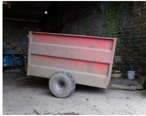
Quad Bike Trailer with Chequer Plate floor with Division Gate & Storage Box
