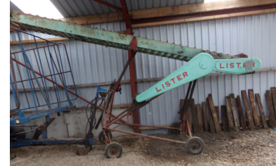
Lister Electric Elevator
